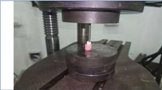
[Table/Fig-2]: Specimens were subjected to a Universal Testing Machine (UTM) to test fracture resistance.
